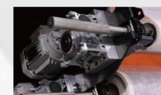
Frequency motor ensures more stable material loading and take-up
