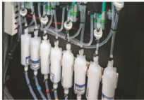
Filter: Combined with negative pressure ink supply system, filtering ink and air impurities
