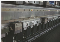
Mute Linear Motor System, no belt, no pvc encoder strip, Increase the Carriage moving precision and Span life
