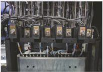
Negative pressure ink supply system: good for long time printing and cleaning
