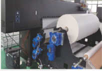
The air shaft media system supports 3000m or 10,000m media roll
